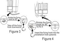
Rotate the drain hose fixing hook for 90 to take it out from the installation hole (As per Figure 3).
